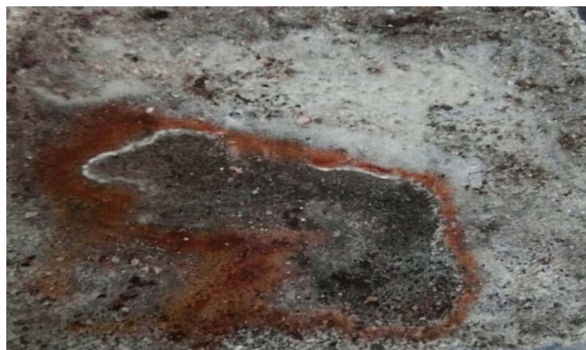
Fig. 2: cement mortar cube attacked by acid.
